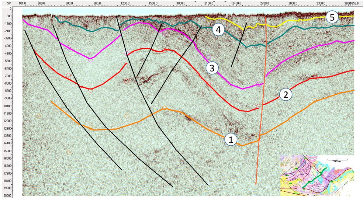
Figure 9. Paleozoic basement (horizon#3) was uplifted in center of seismic section.
