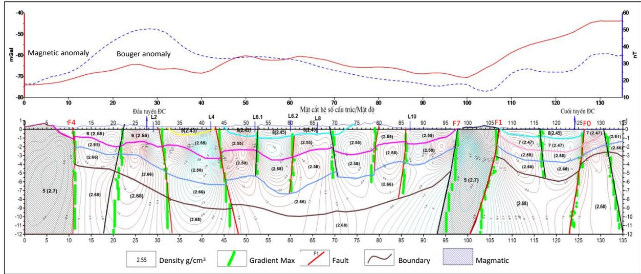
Figure 7. Defining faults and dip direction on Structure-Gravity density-Magnetic susceptibility section.
