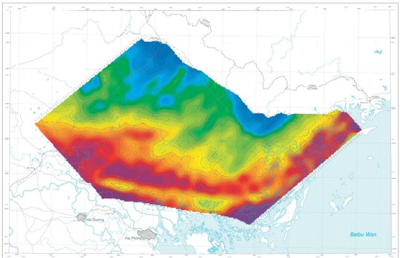
Figure 3a. Gravity Bouguer anomaly Map of An Chau trough.
