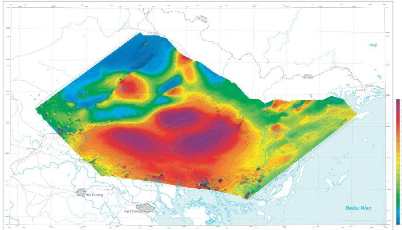
Figure 3b. Total field Magnetic Intensity Map of An Chau trough.
