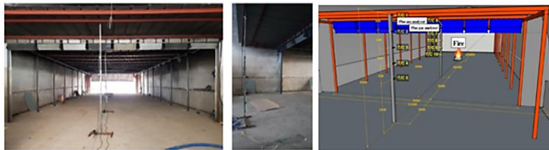
(b) Set up the sensor measurements (T/C and gas analyzer)
