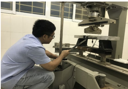
Figure 10. Testing of reinforced concrete sheeting. content.
