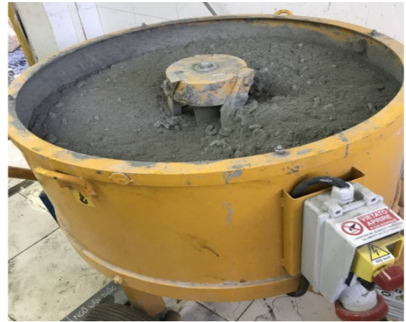
Figure 2. Control concrete mixer.
