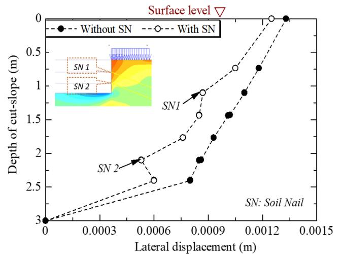
Figure 9. The trend of horizontal displacement of wall face.
