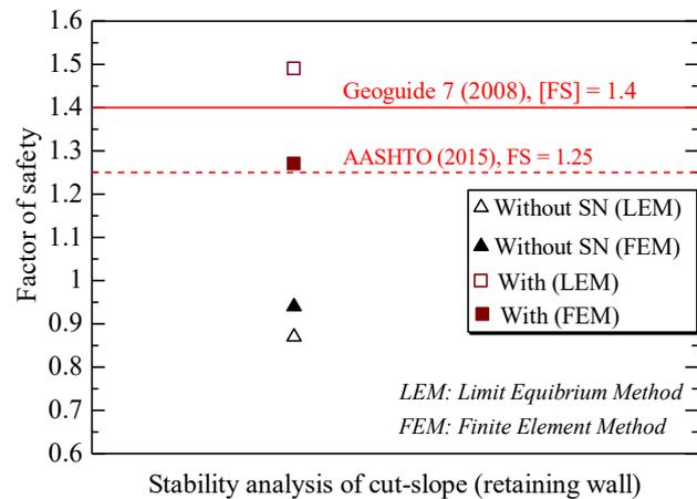
Figure 4. Stability of reinforced wall estimated from analytical and strength reduction methods.
