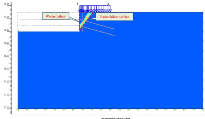
Figure 5. Failure zone in the numerical model.
