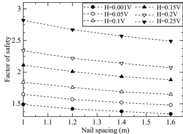
Figure 11. Effect of nail spacing on cut-slope stability.
