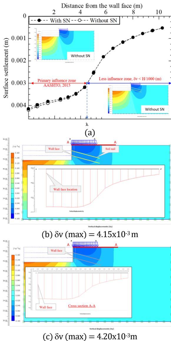
Figure 8. Surface settlement distribution of two scenarios (a), (b) with, (c) without soil nail.
