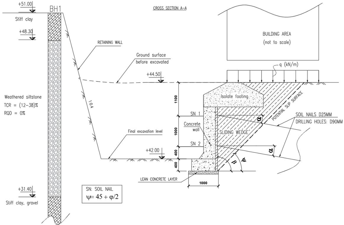
Figure 2. (a) Plan view of shallow foundation; (b) Typical cross-section of ground condition underneath the building.
