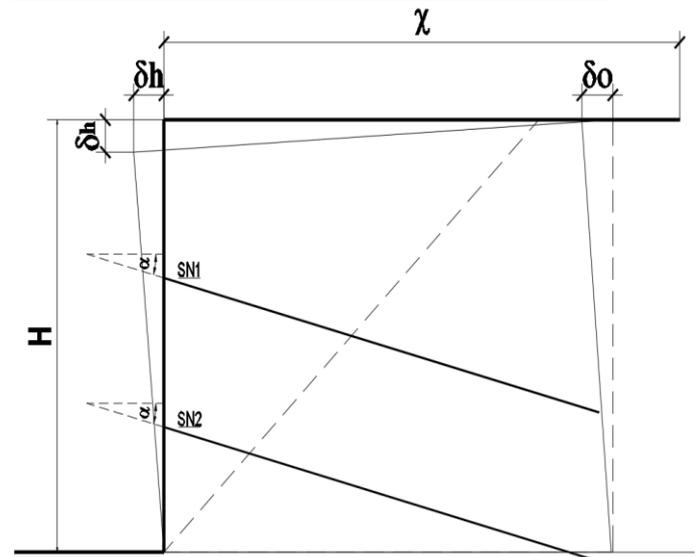
Figure 7. Deformation of soil nailed wall adopted from Lazarte et al. (2015).
