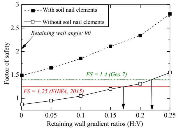
Figure 10. Effects of wall inclination on the stability of the ground.
