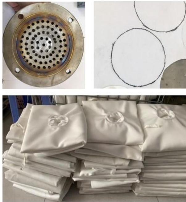
Figure 6. Filter cloth and supporting unit used in filtration test.
