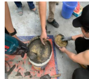
Add steel fibers into the mixed blend
