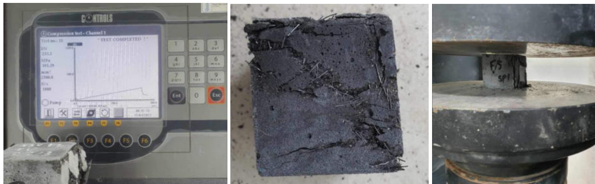
Figure 5. Compression test determining the compressive strength of steel fiber-reinforced concrete.
