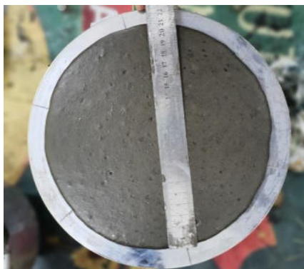
Figure 3. The Experiment measuring the spread flow of concrete.
