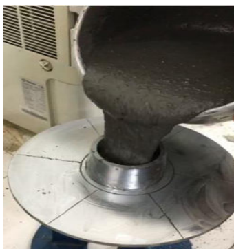
Figure 3. The Experiment measuring the spread flow of concrete.
