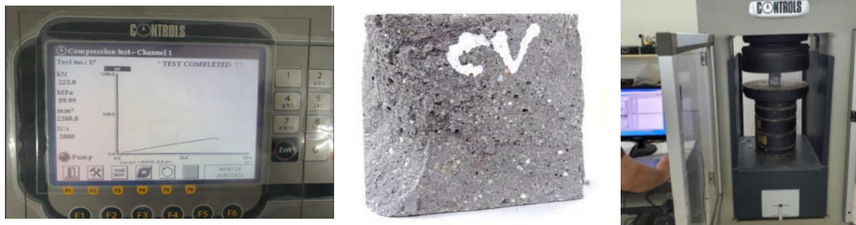
Figure 4. Compression test to determine the compressive strength of concrete without steel fibers.
