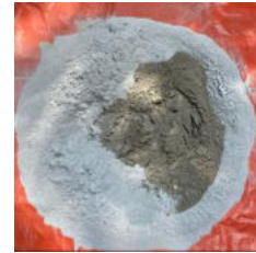
Mix a dry blend of cement and silica fume
