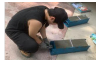
Remove the mold and curing
