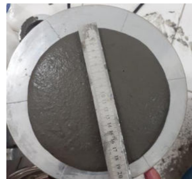
Figure 3. The Experiment measuring the spread flow of concrete.
