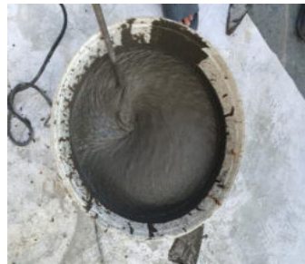
Add superplasticizer into the cement + silica fume mixture
