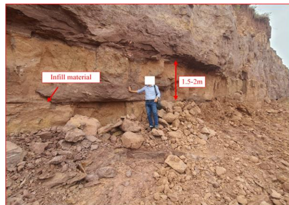
Figure 4. Interbedded siltstone at the head scarp of slope failure Do et al. (2024).
